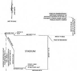
BEARINGS ARE REFERENCED TO THE FLOR-DA STATE PLANE COORDINATE STSTEM, WEST ZONE, KAD B3, 2011 ADJUSTWENT, ESTABLISHING A BEARING OF SOOTD'S STW, ALONG THE EAST LINE OF THE SOUTHELAST QUARTER OF SECTION 2.4, TOWNESHEP 31 SOUTH, BANGE 16 EAST, PHELIAS COUNTY, REGIDA.
